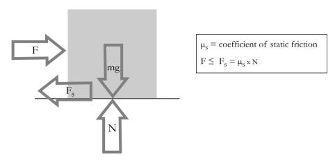
5) Once the force of Static Friction is overcome, the force of Kinetic Friction is what slows down a moving object.
